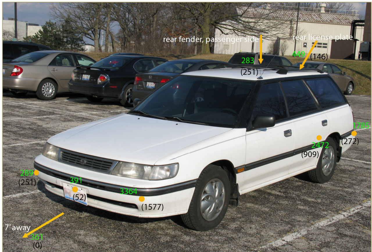
Figure 10 - The results from table 1. The orange dots indicate the location of the magnet. The Walker readings are shown in green for each location, with the PNI readings in black parenthesis.
