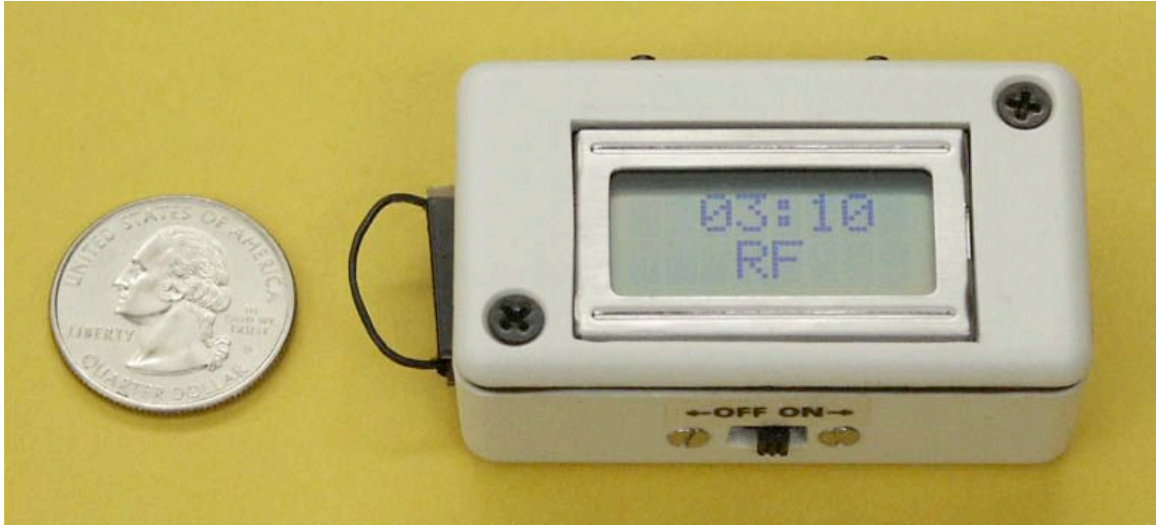
Fig 4 - Prototype Time Trap. When the container is opened, the time trap erases the secret key used by the hash algorithm, and then the time trap shows the time when the container was opened (elapsed or Greenwich Mean Time) and the 2-letter hash associated with that time ("RF" in the photo). In this photo, the container was opened 3 hours and 12 minutes after tamper monitoring began. Like the other (reusable) electronic seals described in this paper, the Time Trap has an adjustable countdown time when first powered up to allow the seal user to close the container or exit the transport vehicle before monitoring begins.
