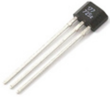
Hall Effect magnetometer, ~$0.85
