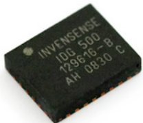
gyro (angular rate sensor), ~$23
