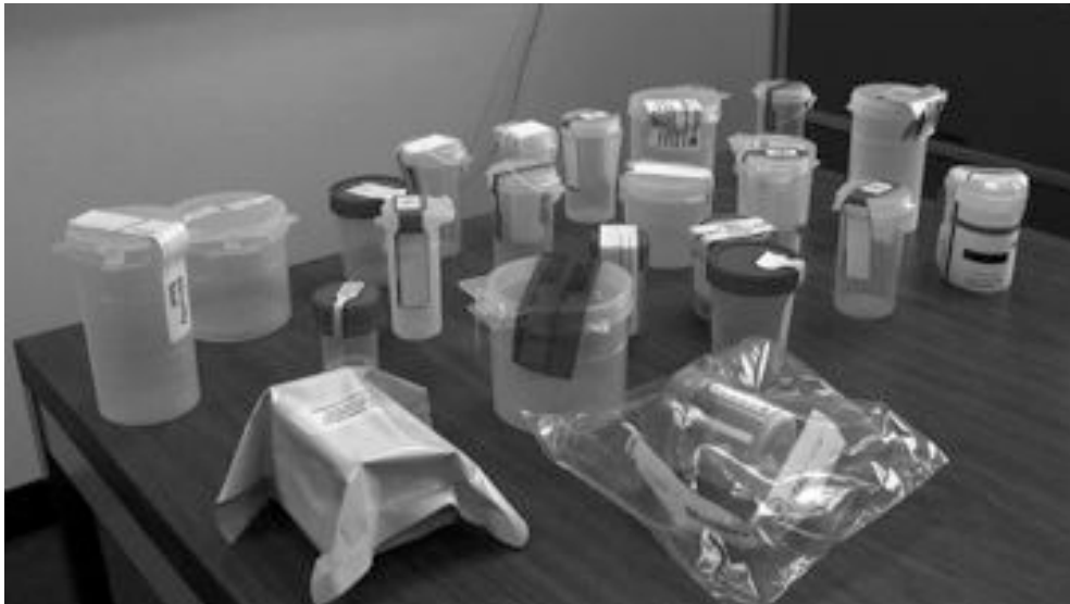
Figure 1 - 22 of the 23 commercial urine drug testing products that were studied. (Figure 3 shows the other product.) Most of the adhesive label seals shown attached to the sample collection vial are meant to be applied after sample collection, but some are meant to detect tampering with the unused sample collection vial.
