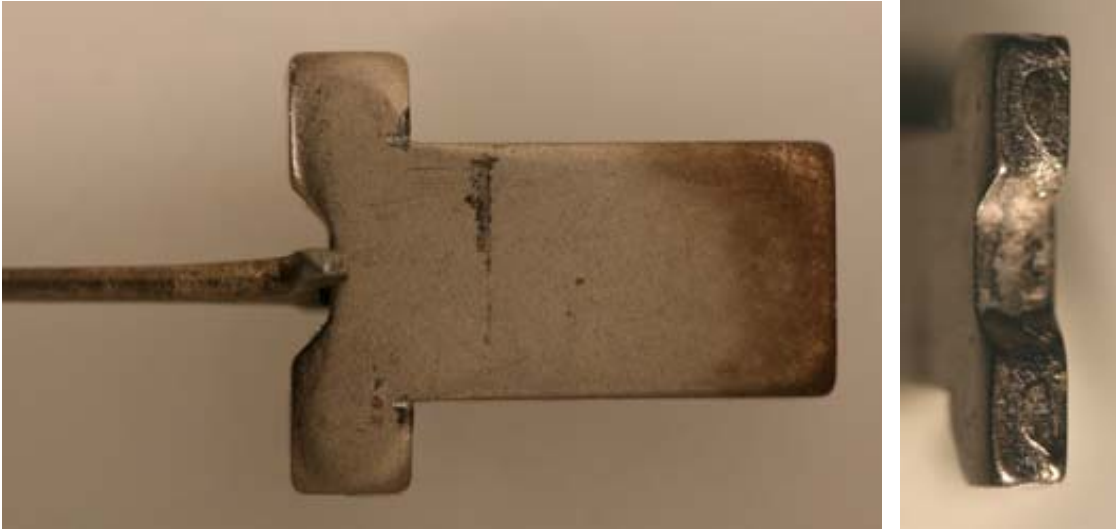
The manipulation tool is formed to precisely grab the edge of the tailpiece that abuts the end of the keyway.
