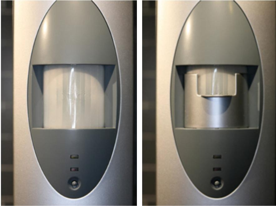
The LaserShield motion sensor can be masked so it is insensitive to pets. The unit on the right has a plastic insert that covers most of the sensing area of the detector so it will not trip from small animal movement.
