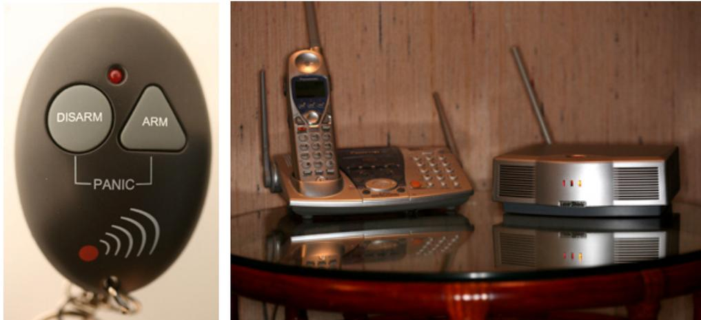
A wireless key fob controls the entire system. This device has a fixed code that can be cloned with the proper equipment and expertise<sup>2</sup>. Normally the master alarm unit is located in a convenient location so the internal panic button can be activated in an emergency.
