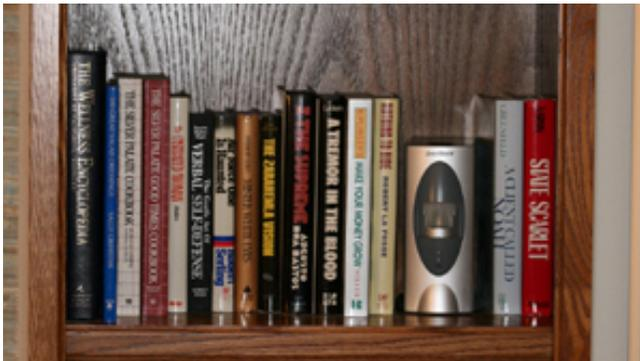
**A LaserShield Passive Infrared motion sensor is inconspicuously placed in a bookcase.**
