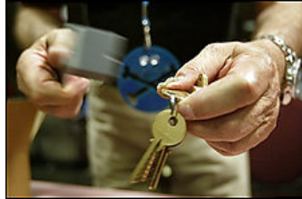
Marc Tobias demonstrates a bumping technique to open a post office lock during DEFCON 14 at the Riviera in Las Vegas on Saturday, Aug. 5, 2006. Tobias, a South Dakota lawyer who authored a textbook for locksmiths, showed how a simple technique can allow a person to secretly pick the locks of most homes, businesses and post office mailboxes. (AP Photo/Jane Kalinowsky) (Jane Kalinowsky - AP)
