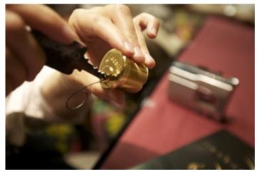
A Medeco mortise cylinder with a bent paper clip and plastic key.
