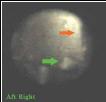
Advanced decoding with an Olympus borescope provides information about the bottom pins. This information can be used to open Medeco locks.
