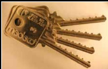
Four code setting keys can be used to open virtually every non-master keyed Medeco Biaxial and m3 cylinder that was produced prior to December 2007.
