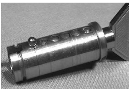
Figure 2.39: Maxis plug with pins at shear line.
