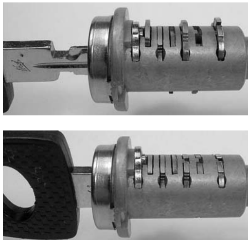
Figure 7.30: Operation of Mercedes four-track lock.
