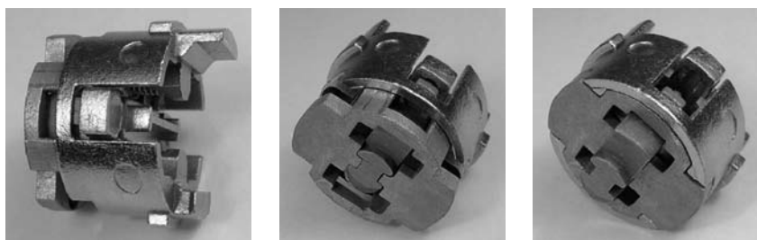
Figure 5.130: Rear section of Fichet 787 core: (left) side view showing cross-piece and fence; (middle) tail-piece retracted; (right) tail-piece extended.
