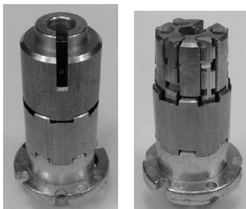
Figure 3.58: (Left) Laperche core. (Right) With cover removed.
