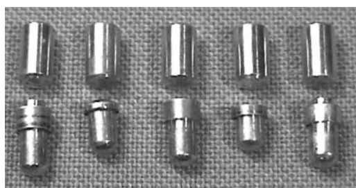
Figure 2.40: Set of lower pins and drivers from Maxis cylinder.
