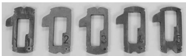
Figure 7.22: Wafers from Mercedes two-track lock.
