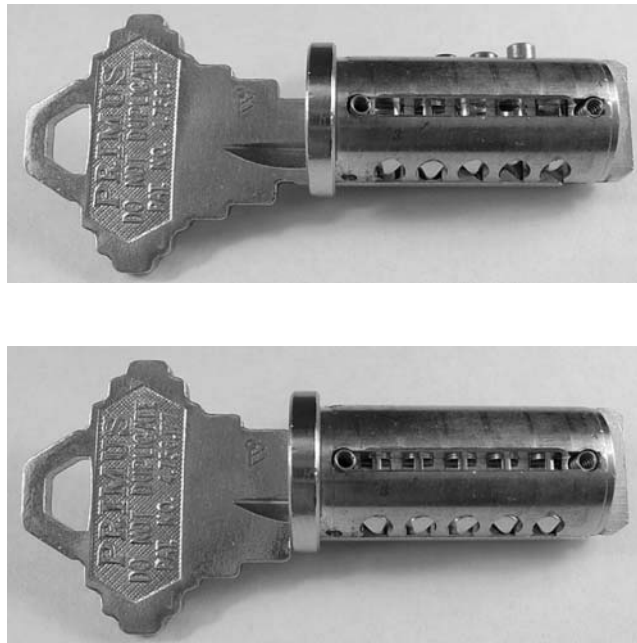
Figure 4.118: Operation of Schlage Primus core with side-bar removed: key aligns finger pins.
