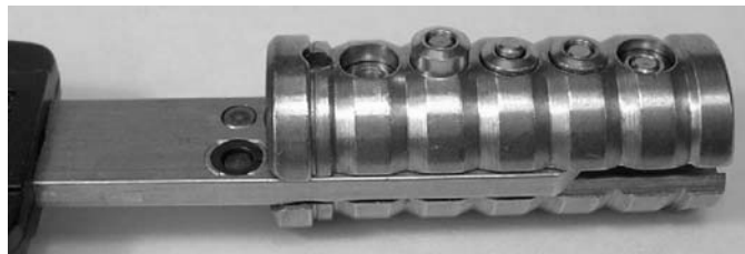
Figure 2.191: Key partially inserted: movable insert not yet in contact with pin 1.
