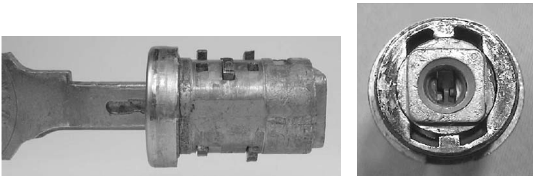
Figure 3.37: Key insertion: side tracks pick up bar-wafer stumps.
