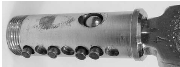
Figure 6.17: Miwa EC plug with key inserted (magnets reversed for photo).
