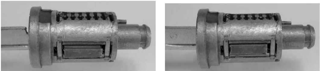
Figure 7.18: GM plug in locked position (left) and with side-bar retracted (right).
