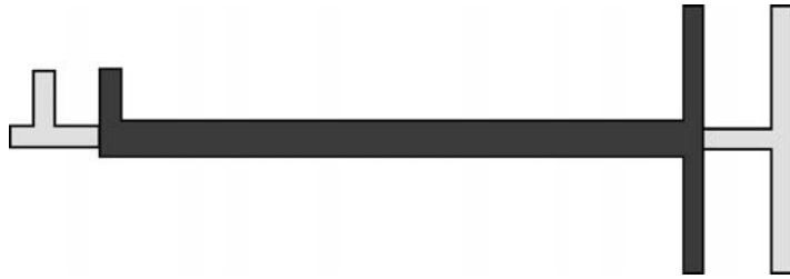
Figure 1.11: A two-in-one or Hobbs pick for manipulating lever locks.
