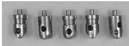
Figure 4.59: Medeco cam lock pins with either false-depth hole or antipick groove.
