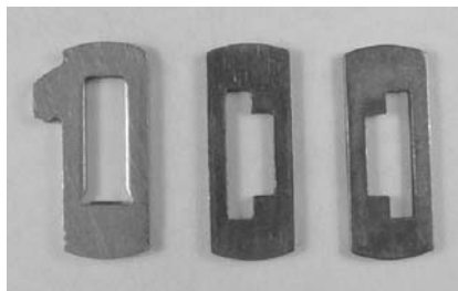
Figure 3.18: Conventional wafer-tumbler and two Bricard wafer-tumblers.
