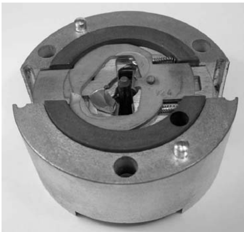
Figure 5.117: Kromer BP55K lock with front cover off: (left) curtain plate removed to show lever pack; (right) operation by correct key.
