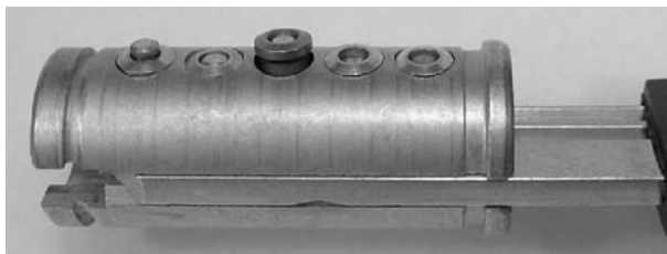
Figure 2.186: Mul-T-Lock plug with key partially inserted.
