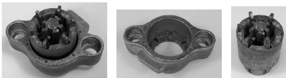
Figure 3.53: Supra 6-slider core and rear cap.
