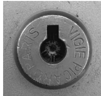
Figure 3.61: Front and rear keyway of a Vigie Picard lock.
