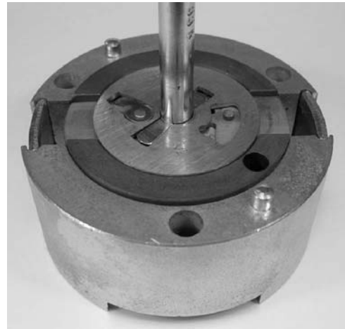
Figure 5.117: Kromer BP55K lock with front cover off: (left) curtain plate removed to show lever pack; (right) operation by correct key.
