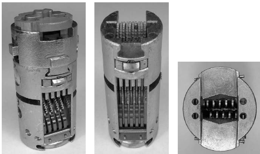
Figure 5.129: (Left) Fichet 787 core. (Middle) Core with rear section removed to show gears. (Right) View through gates at front of keyway.
