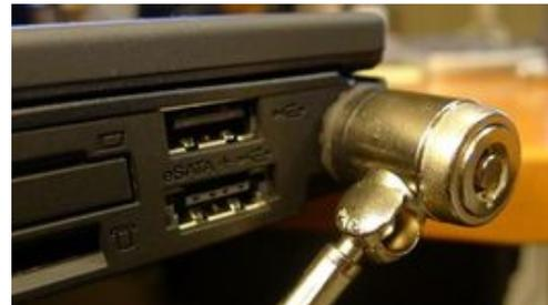
This is the HP cable lock attached to a Lenovo laptop. It can be removed in seconds by rapping the... [+]
