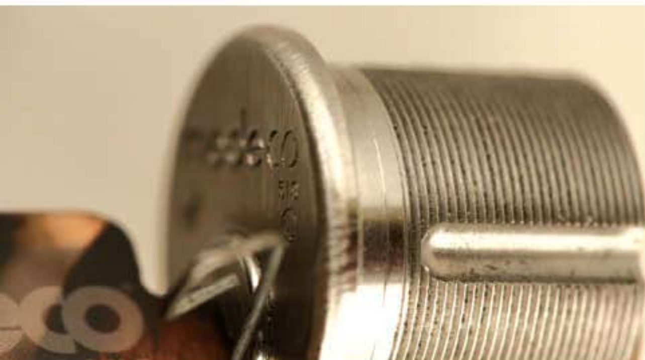
The most popular high security lock in America can be easily bypassed by the use of a simulated key, produced from a plastic credit card. This lock contains three separate layers of security. The plastic key bypasses two of them, and the paper clip circumvents the third element.
